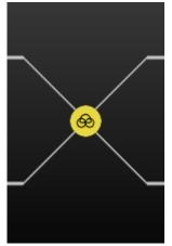
The Mid-Side module can be used to encode a Left/Right input to Mid/Side, or decode a Mid/Side signal to Left/Right. This is useful for Mid/Side signal monitoring, accessing the Mid/Side signal components independently, or using Mid/Side recordings in a traditional Left/Right stereo context.
