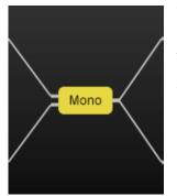
The Mono module inserts a mono switch into the signal path. Activating the mono button adds the two channels together.
