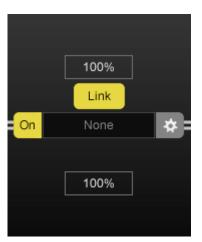
The Wet/Dry controls will be shown when a plug-in slot is on. They can be used to blend the incoming signal with the output signal processed by the Insert effect. 0% is completely dry and 100% is completely wet. The Link control is only available in stereo mode and links the value of the Wet/Dry mix for each side.
