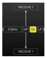
The Crossover module allows the signal to be split at a specified frequency, with the signal above or below the crossover point (depending upon the filter chosen) passing through for further processing.
